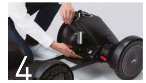
4 Pull the lever on the side of the battery toward you to separate the parts.
